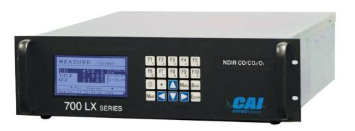
CAI ENVEA Group's 700 LX NDIR O2 Analyzer measurements are based on the infrared absorption characteristics of gases. Using a single infrared beam to measure gas concentrations, they deliver highly stable and reliable results.
